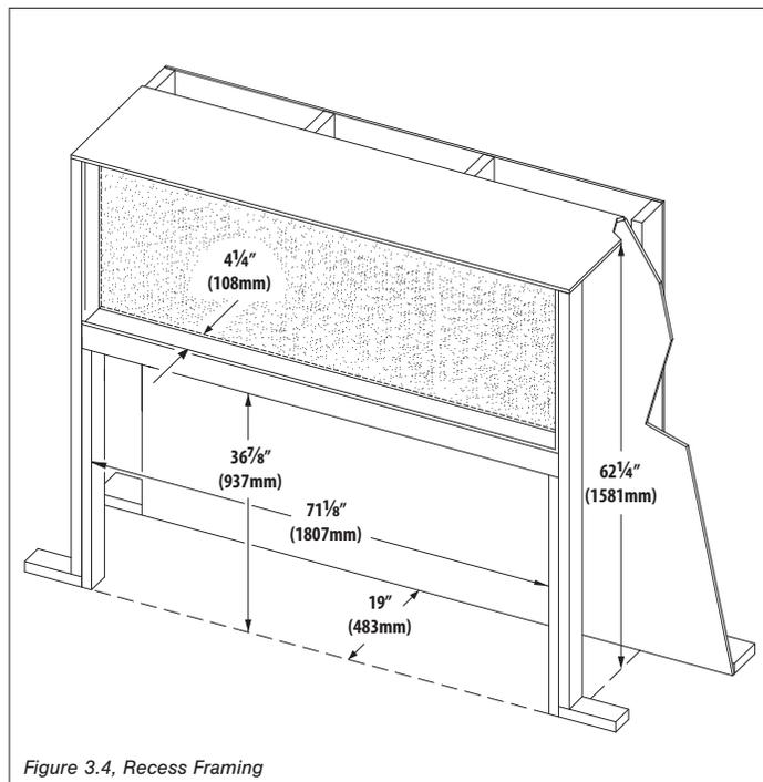
Figure 3.4, Recess Framing
