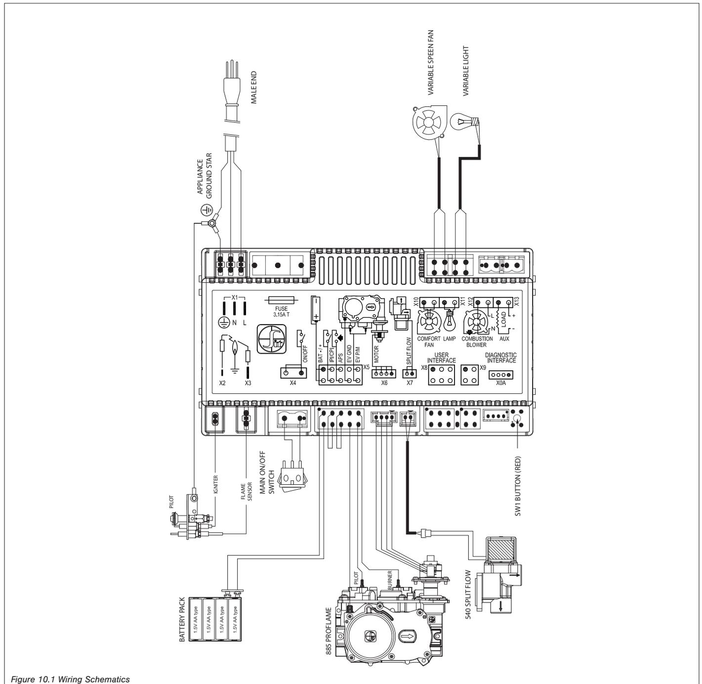
Figure 10.1 Wiring Schematics
