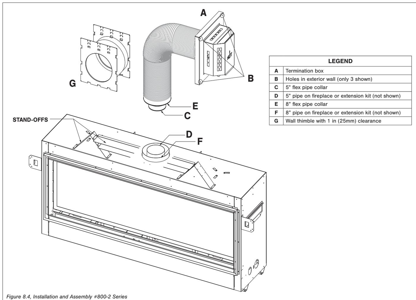
Figure 8.4, Installation and Assembly #800-2 Series
