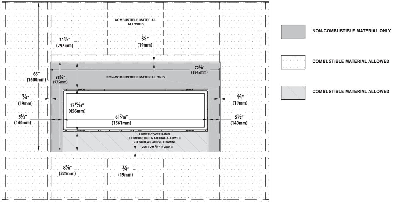
Figure 5.3, Minimum Non-Combustible Material Dimensions
