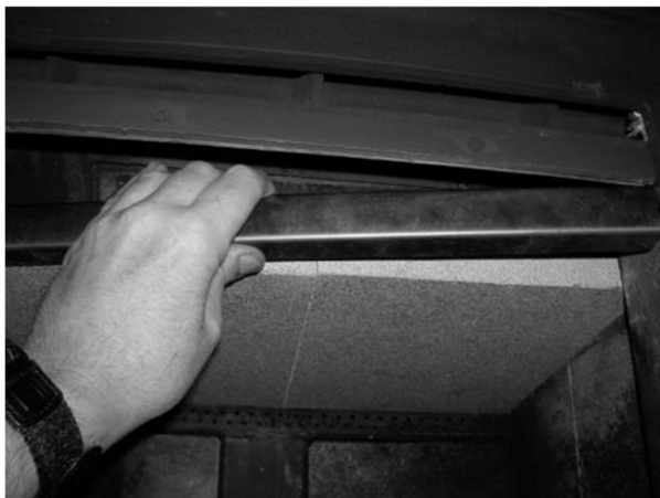
Figure 19a – Removing / Replacing the Baffle
