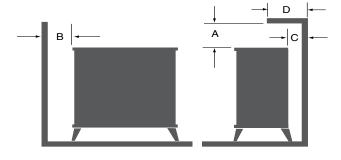
Vermont Castings direct vent gas stoves must be installed on rigid flooring. When the heater is installed directly on any combustible surface other than wood flooring, a metal or wood panel extending the full width and depth of the unit must be used as the hearth.
