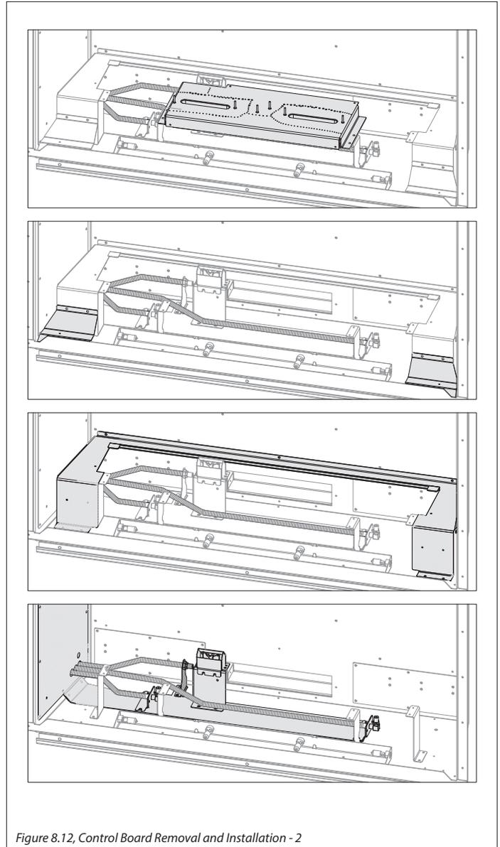
Figure 8.12, Control Board Removal and Installation - 2
