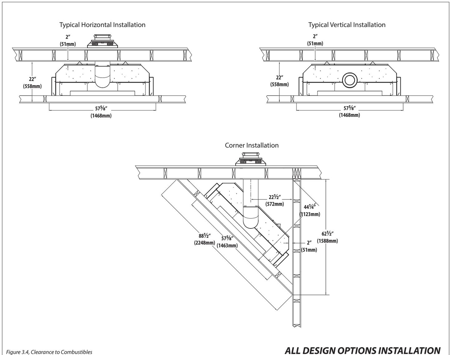
Figure 3.4, Clearance to Combustibles
