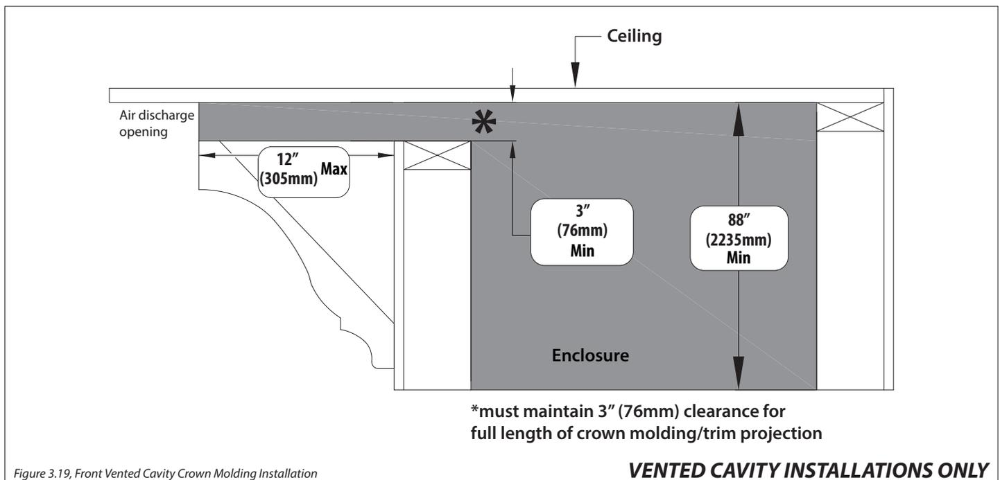
Figure 3.19, Front Vented Cavity Crown Molding Installation
