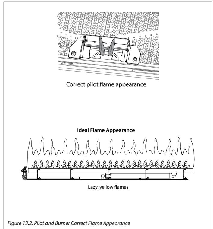
Figure 13.2, Pilot and Burner Correct Flame Appearance
