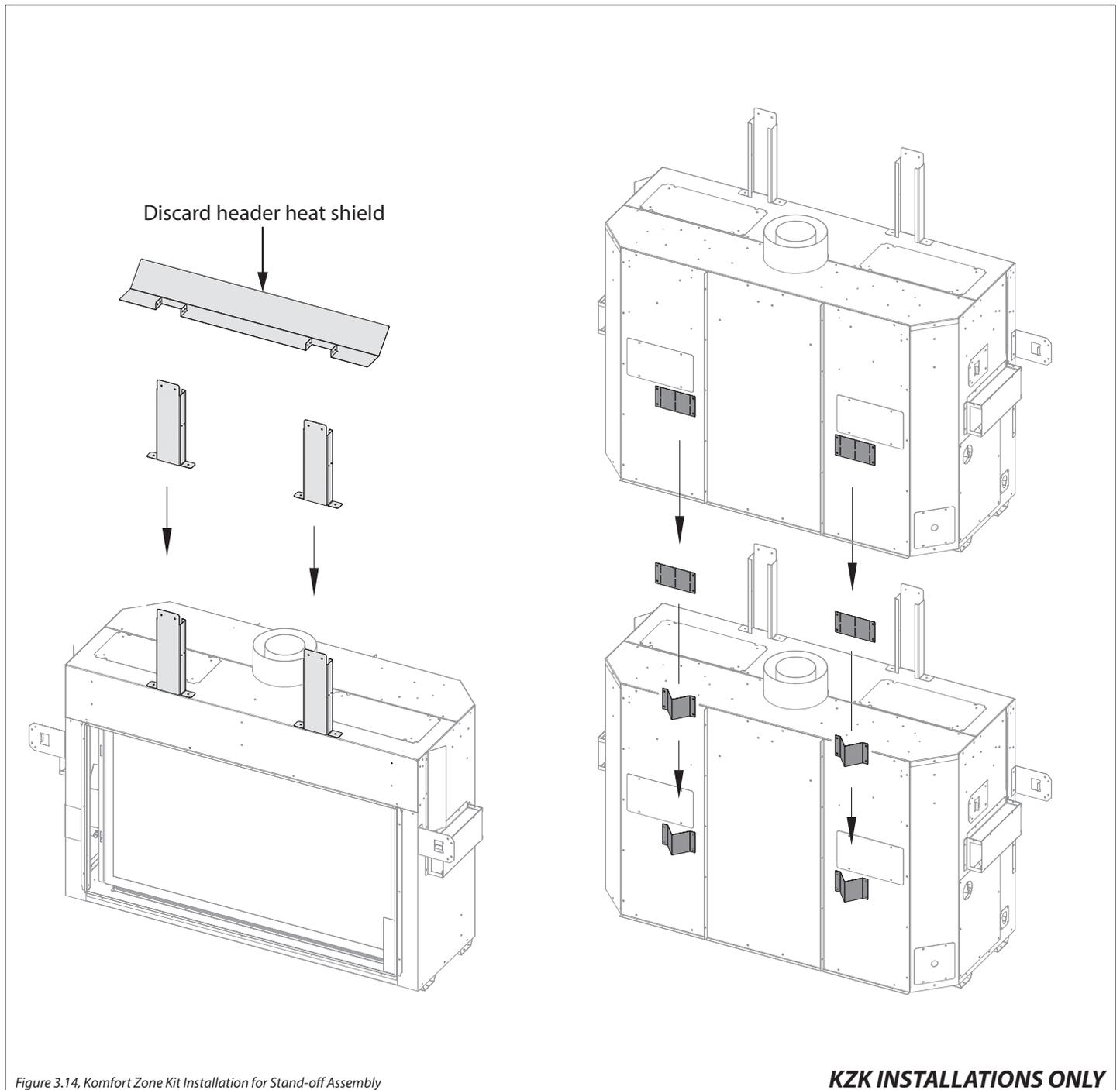
Figure 3.14, Komfort Zone Kit Installation for Stand-off Assembly
