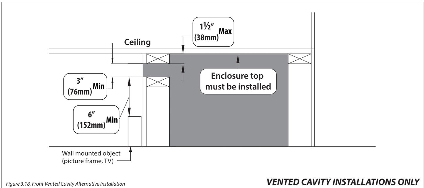
Figure 3.18, Front Vented Cavity Alternative Installation
