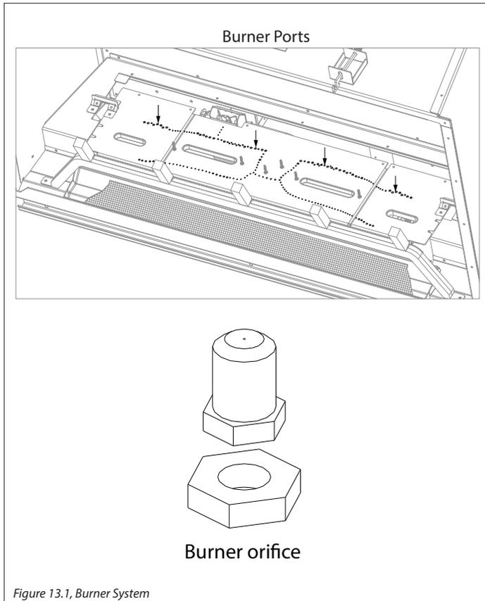
Figure 13.1, Burner System
