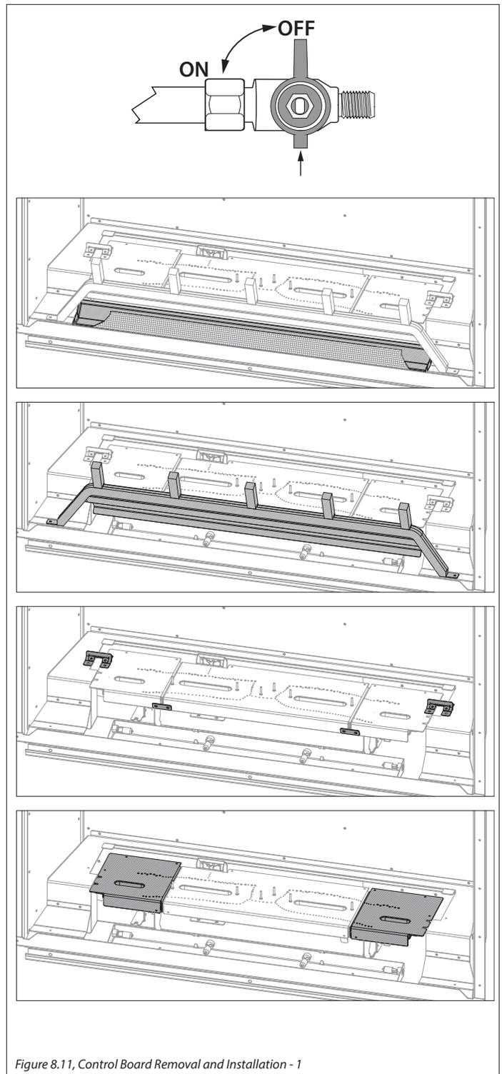
Figure 8.11, Control Board Removal and Installation - 1
