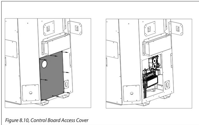
Figure 8.10, Control Board Access Cover
