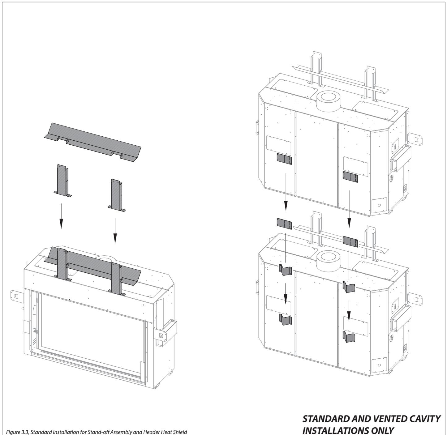
Figure 3.3, Standard Installation for Stand-off Assembly and Header Heat Shield
