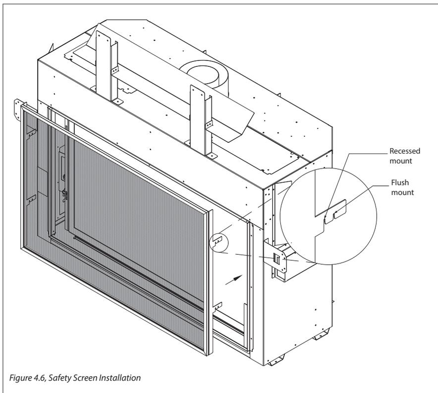
Figure 4.6, Safety Screen Installation
