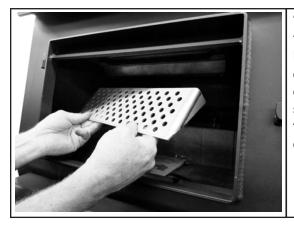
**7.** Once the combustor is installed completely so that all three tabs at touching the face of the dome, replace the flame shield. Note the flame shield sides are shaped like a triangle. The point of the triangle should face down when installed correctly. Never operate your stove without the flame shield in place. The flame shield will protect the face of the combustor against damages from wood when loading and other possible damages that can occur during the cleaning process.
