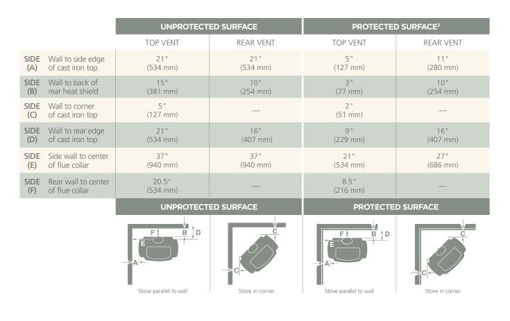
Using listed double wall oval to 6" or 8" round connector; all installations require supplied rear heat shield, flue collar shield and bottom heat shield.
